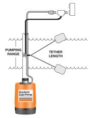
Pumping range determined by tether length according to the following guide.
